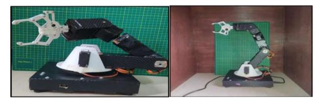
In the current design, configuration and parts used, the arm has a maximum load capacity of 200 gm when fully extended. The cost of the entire project was also minimized and kept under ₹10,000.
