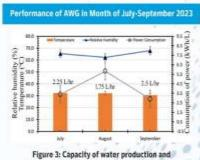
Figure 3: Capacity of water production and Power consumption at various conditions in month of July-September 2023
